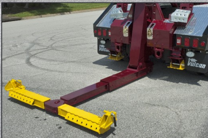
The V-24 comes standard with a low-profile crossbar with removable ends, one set of lift forks, fork holders and a 6,000-lb. Vulcan Wheel Retainer System.
