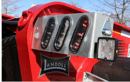
Optional Stop Tail Turn with Work Light Gooseneck Mounted
