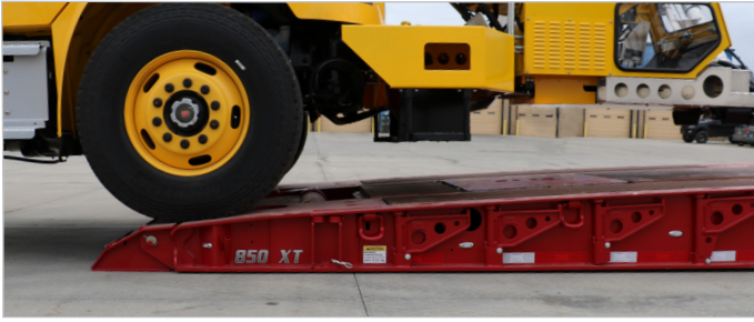
Pin-On Assist Ramp with Traction Bars and Keyhole Tie Downs on Approach
