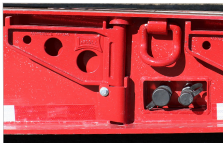
Angled D-Rings, 12" Swing-Out Riggers, Secondary Locations for Hydraulic Quick Couplers
