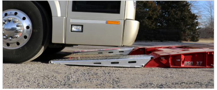
Pin-On Assist Ramp with Traction Bars and Keyhole Tie Downs on Approach
