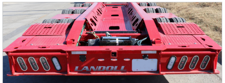
Four Light Combo – High Visibility LED Lights, Stop-Tail-Turn Strobe (STD)
