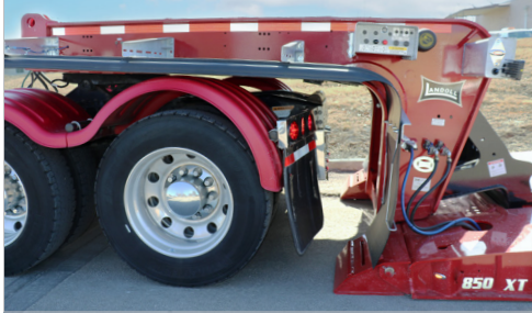
Easily Adjust Ground Clearance from 6" to 20"
